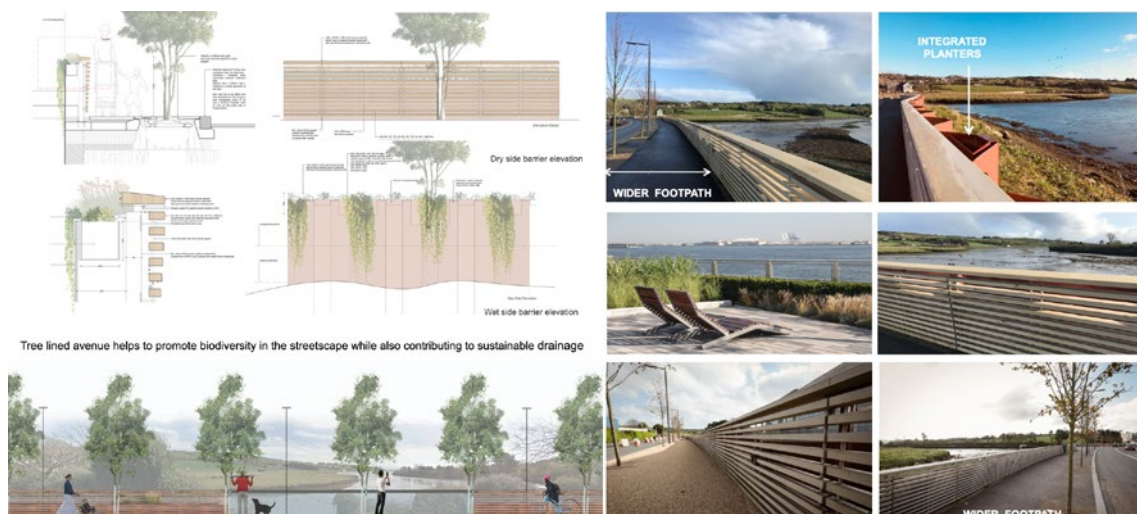
Flood-defence walls along the banks of the River Fealge were replaced and repaired. The design of new areas of construction improved the public space with widened footpaths, enhanced wall finishes, quality architectural lighting and landscape features. Clonakilty 400 Urban Design Masterplan (case study 19), Ireland. Courtesy of Cork County Council architect Giulia Vallone
